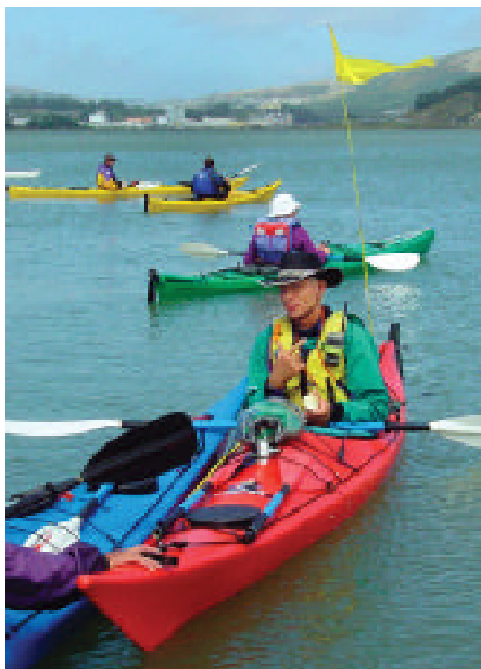
Brightly coloured kayak and lifejacket. Spare split paddle on foredeck; VHF radio on the lifejacket; high visibility 'chopper' guard flag on the stern.
