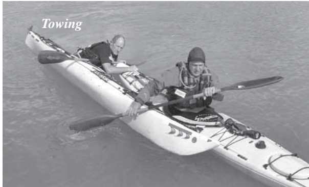
For a short distance, a contact tow provides support for a sick or injured paddler. A short line connects the towed kayak's bow to the foredeck of the towing kayak, so the tower can still paddle
