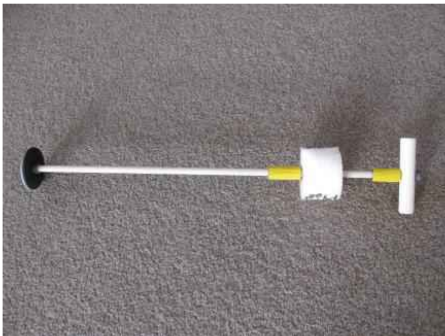
Shaft assembled with piston, flapper, bottom spacer, float, top spacer, handle
