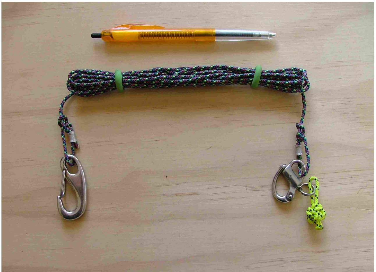
The finished lightweight rescue line, snap hook to left and snap shackle to right
