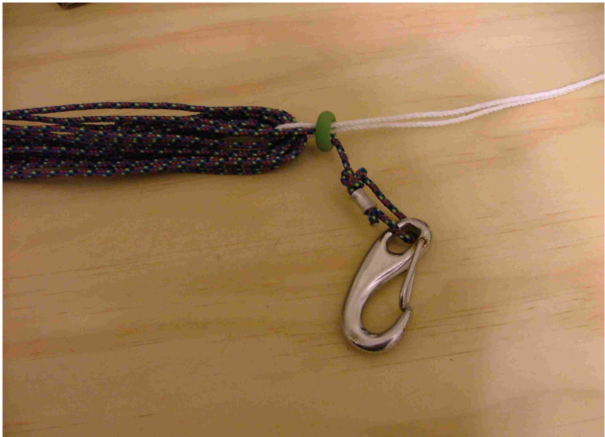
Use a loop of spare line to ease the loops through the rubber ring
