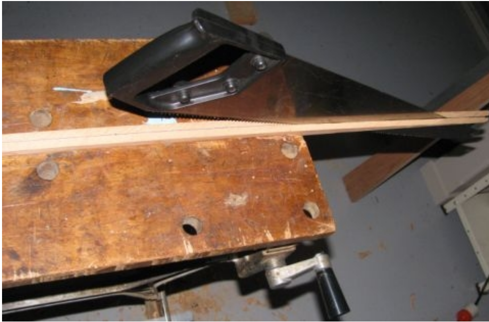
Splitting the offcuts
