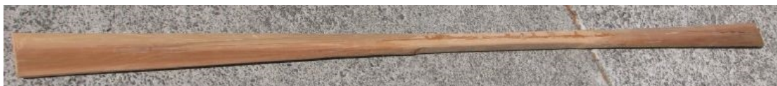
The paddle has been shaped and it is just possible to see the glue lines. Note that the pieces glued on are now shaped back by at least a third of the length of the blade.
