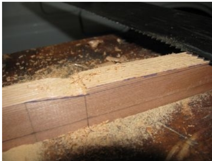
The rough shape of the paddle has been cut. The loom is now being roughly cut to shape
