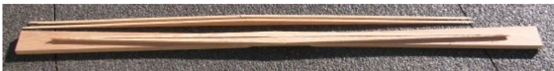
One of the split pair on the paddle where it will be glued (Storm paddle)
