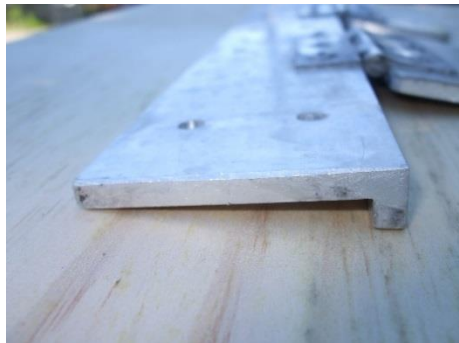
Extrusion section showing hinge and nib relative positions
