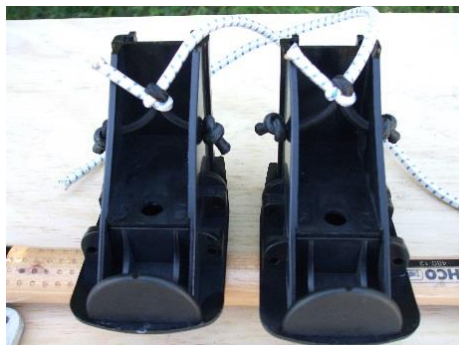
New shock cord added to original
