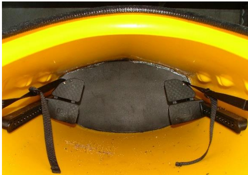
Typical OZO footrest arrangement
