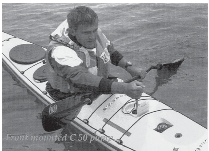
Figure 10) A front mounted pump is easier to use than a rear deck pump, but it does take away from your space under the deck.
