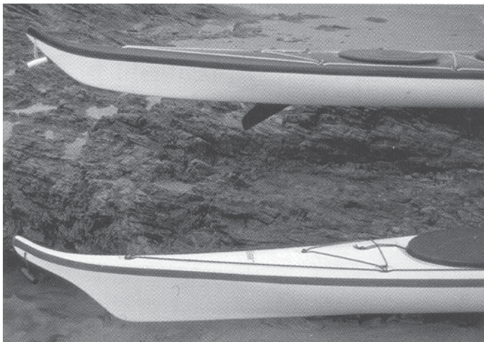
Figure 1) A single change on the hull can totally change the handling characteristics of the boat. Top boat; Nordkapp H, Bottom boat; Nordkapp HM.
